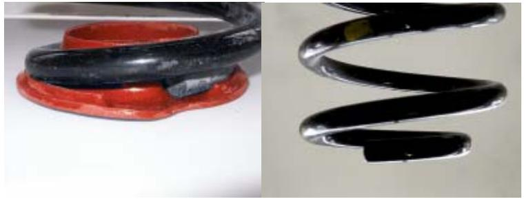
Note that there is little support under the coil as it rises from the urethane seat. Also, one can see that the distal end of the coil is lower than the side 180° opposite. Sand, dirt and other road grit will accumulate in this low area as the spring flexes up and down, creating an abrasive condition that promotes wear. Even when the spring is under full compression, the vehicle's weight is not evenly distributed the over the seat.
