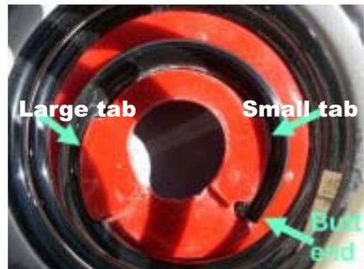
These tabs hold the seat on the spring and prevent it from rotating. **Do not cut them off.** With the spring on a stable surface, lined up the end of the spring coil (both ends are the same) with the space provided on the seat, as indicated by the green arrow "Butt end", and insert the larger seat tab under the spring coil. Press down on the seat so that the small tab snaps over the coil.
