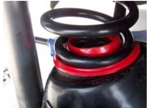
Place the lower, "hat" shaped seat in its original location on the suspension arm with "notch" facing toward the front of the car. Actually, there is only one way to set the seat due to the shape of the steel retainer.
