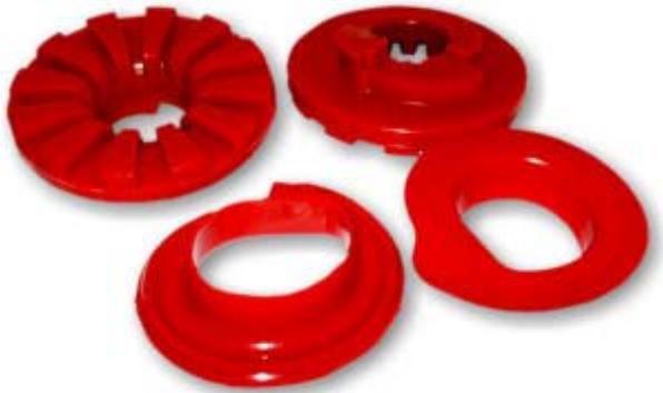
Your spring seats have been made from custom molded urethane rubber with these specifications; 90 Shore A hardness, 300 pli (pounds per linear inch) tear strength and 600% elongation at break.
