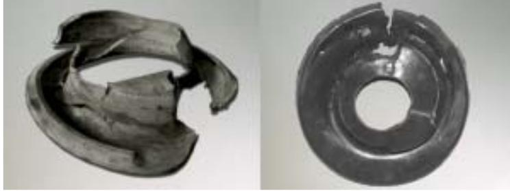
This is normal wear and tear for these parts. They take a real beating, especially if you live in an area with poor roads of speed humps.
