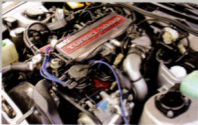
All-new VG30 V-6 engine was good for 200hp in turbocharged trim; 1984 models had an oil-cooled turbo, but later ones were watercooled.
