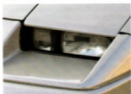
Half-hidden headlamp was a sealed beam with inset fog lamp until 1986; 1987-up models had only the headlamp up top, while the fog lamp moved into the front fascia.
